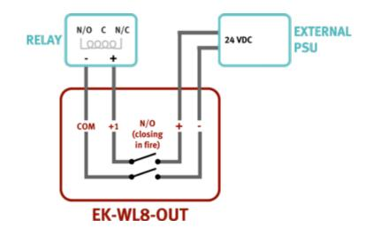
The external PSU will supply the voltage to the power terminals of the Ekho Output Module (rated for 250 VAC but we would recommend only using VDC). When the fire alarm is activated, the Output Module will switch the voltage by closing the two contacts.
